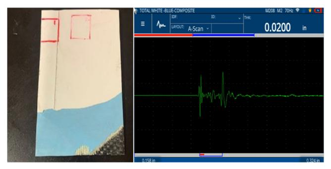
**Individual layer thickness**: In this measurement, the 20 MHz transducer and ultrasonic setup are optimized to amplify the echoes for each of the three layers of the coating on the composite. The coating includes a surfacer layer and two topcoat layers.
